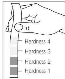
The keys allow you to change the set options: hardness 1 (very soft), hardness 2 (soft), hardness 3 (medium), hardness 4 (hard).
